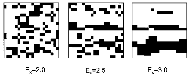
Figure 8 Calculated structures with desired x -elastic moduli (white: component A, black: component B).
